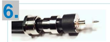
Slide teflon isolator over the center conductor to stop. Then put center pin cautiously on center conductor.
