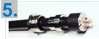
Remove foil and dielectric with a knife. The center conductor must remain absolutely round, if necessary bend carefully.
