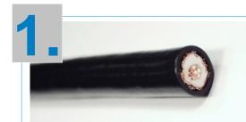
Cut the cable end perpendicularly with a small metal saw. The center conductor must remain absolutely round.
