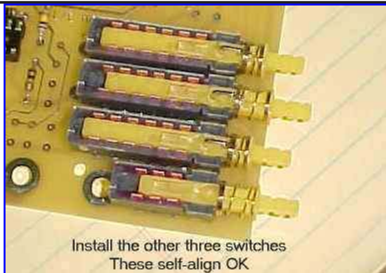
Install the remaining three switches.
