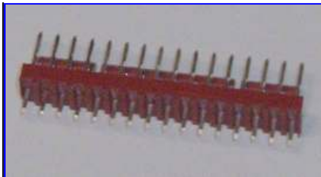
If you received a 14 pin connector install it in pins 1-14 of the PCB. The 16 pin shown is the current production.
