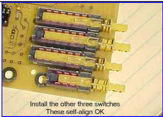
Install the remaining three switches.
